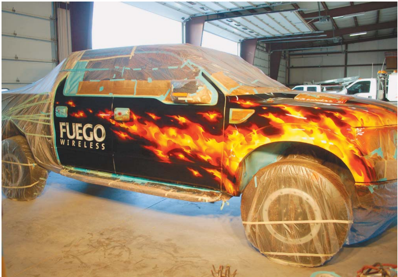
Plastic sheetting is a must when doing painting projects that do not involve disassembling the vehicle.
